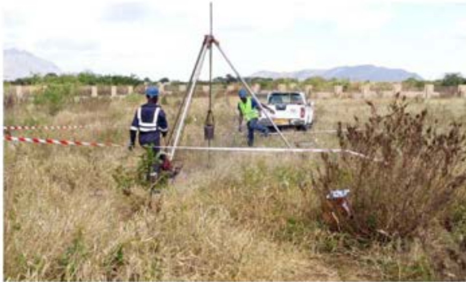
Figure 5-2 –Selected DPSH photo at proposed Kihonda Mini Bus Stand
