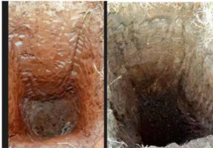
Figure 5-1 – Selected trial Pit (TP 3 & TP 4) photos at the proposed Kihonda mini bus stand.
